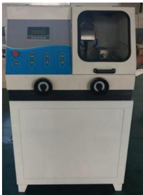
Q 1 0 0 B Automatic Metallographic sample cutting machine
